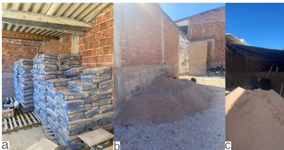
Figura 19: Cimento Portland CP V ARI RS (a), Pó de pedra (b), Areia (c)
